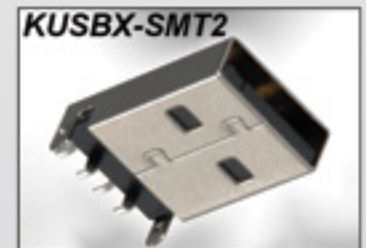
Surface Mount A-Type Plug
